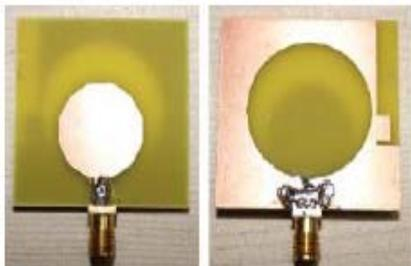
Fig.14: Polygonal-shaped antenna [31]
