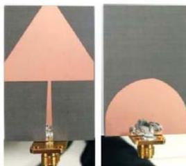
Fig.16: Trapezoid shaped patch antenna with semicircular ground plane [32]
