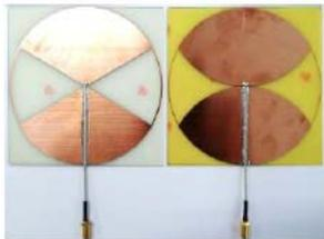
Fig.7: Circular coupled sectorial loop radiator for SWB applications [9]
