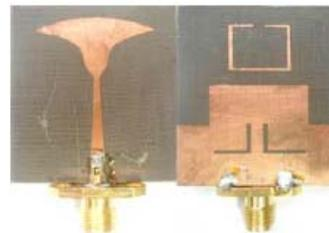
Fig.10: Tapered radiating patch with chamfered ground plane band notched SWB antenna [24]
