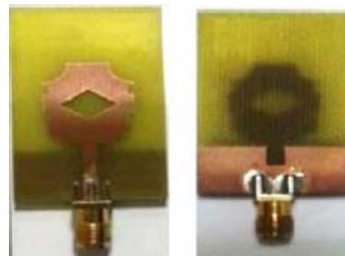
Fig.6: Hut-shaped antenna [8]
