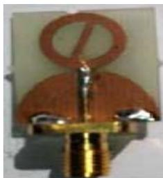
Fig.9: CPW Fed-Phi-shaped patch antenna [20]
