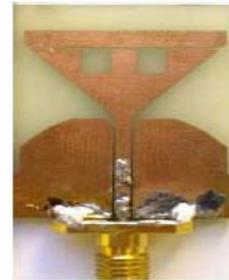
Fig.8: CPW fed inverted triangular shaped patch antenna [13]
