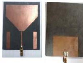
Fig.12: Bevel shaped patch radiator [28]
