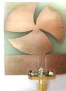
Fig.5 : Propeller shaped monopole radiator with CPW feed [7]
