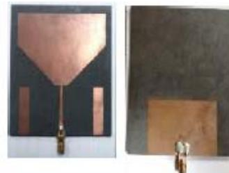
Fig.12: Bevel shaped patch radiator [28]
