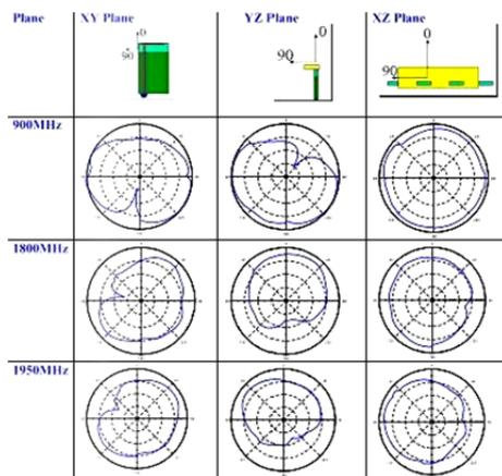
Fig.1. Radiation diagrams of the transmitting antenna.
