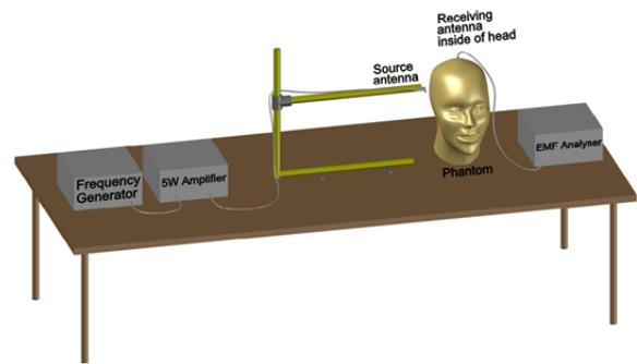
Fig.2. RF exposure system design.
