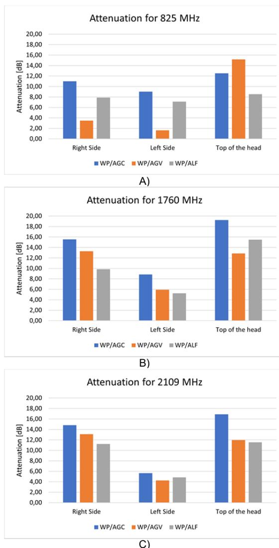
Fig.5. The effectiveness of the attenuation accessories for each side of the head and for frequency A) 825 MHz, B) 1760 MHz, C) 2109 MHz.
