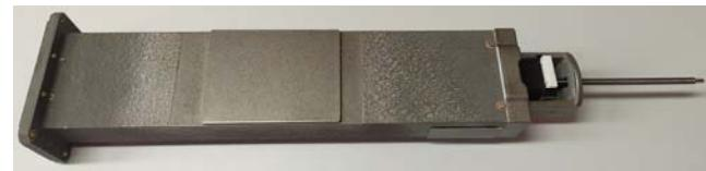
Fig.11. Tunable waveguide shunt connected to linear actuator
