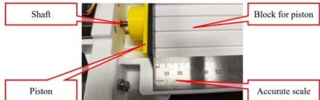
Fig.10. Detail of measurement scale
