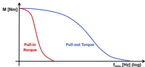
Fig.1. Torque characteristics of stepper motor
