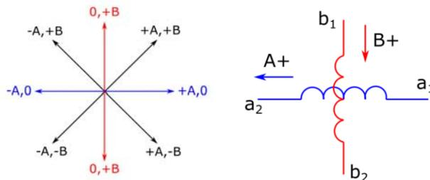
Fig.3. Representation of windings, currents and magnetic field for bipolar stepper motors
