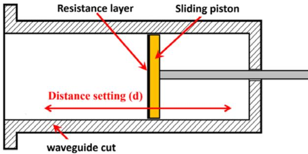
Fig.4. Tunable waveguide shunt
