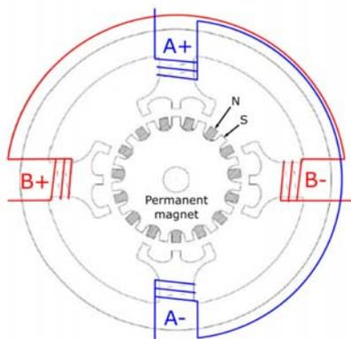
Fig.2. Hybrid stepper motor
