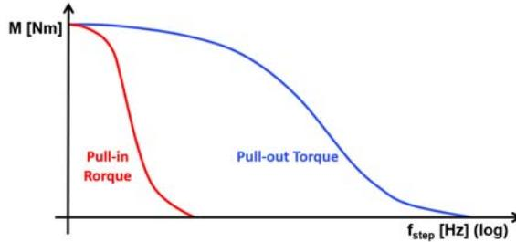
Fig.1. Torque characteristics of stepper motor
