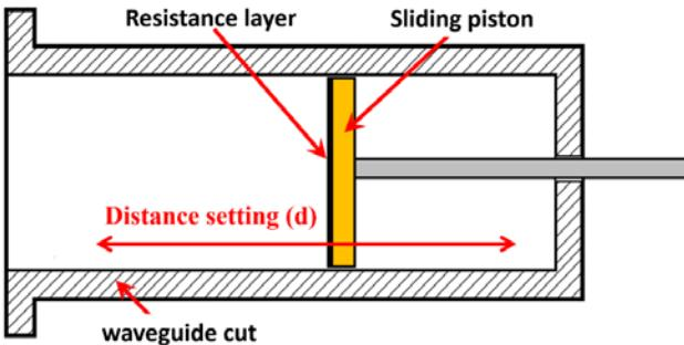
Fig.4. Tunable waveguide shunt
