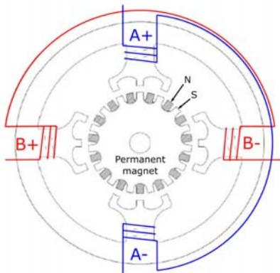
Fig.2. Hybrid stepper motor
