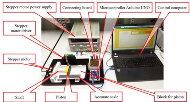
Fig.9. Testing station for precise stepper motor control
