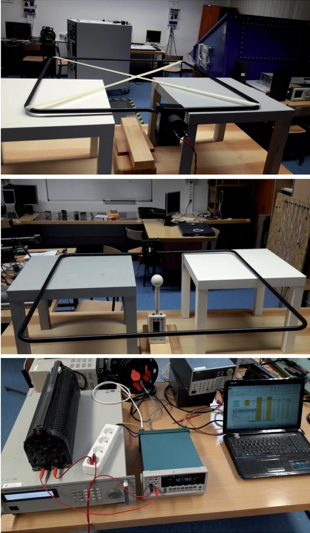
Fig. 3. Set-up for evaluation of the coil factor from top to bottom: marking the coil centre, positioning of the probe, power source and the amperimeter
