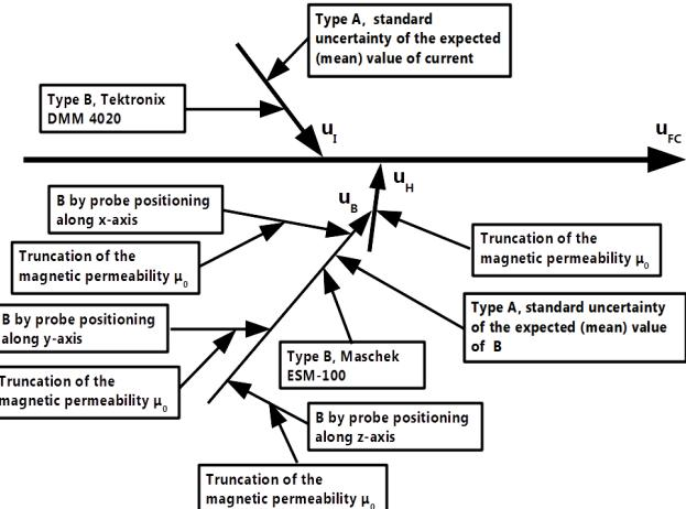
Fig. 6. Fishbone diagram of the uncertainty budget.
