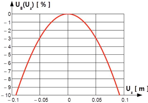
Fig. 4. Maximal error by positioning along symmetry z-axis.
