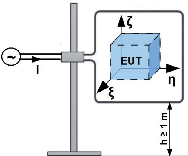
Fig. 1. Set-up for immunity test against power frequency magnetic field.
