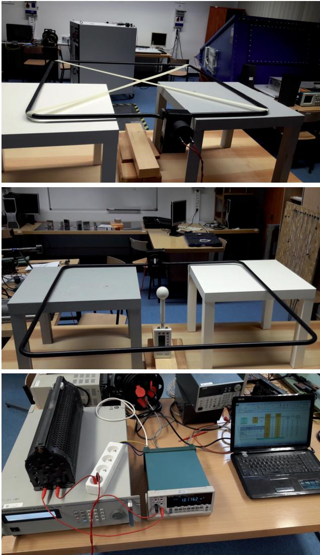
Fig. 3. Set-up for evaluation of the coil factor from top to bottom: marking the coil centre, positioning of the probe, power source and the ampermeter
