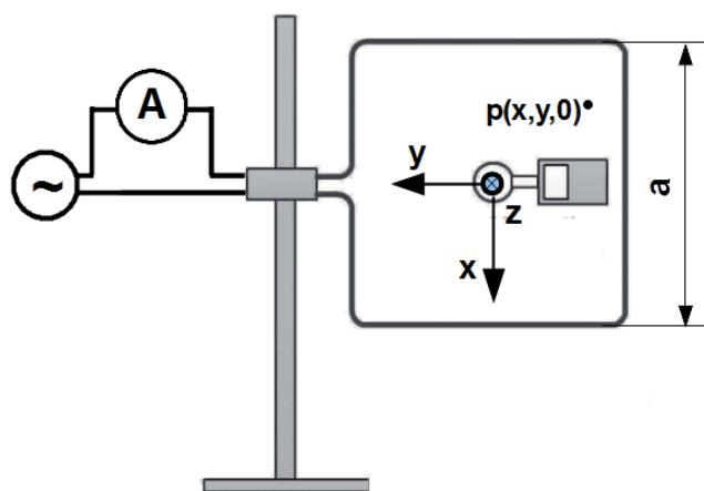
Fig. 2. Set-up for establishing the coil factor.
