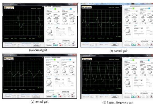
Fig. 3. Generated voltage from PZT placed in a foot with different gait frequency
