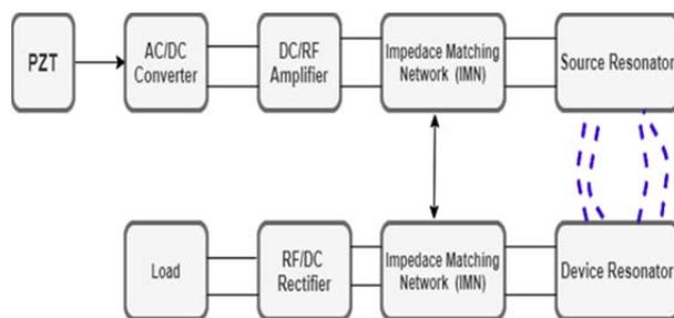
Fig.1. Block diagram of a wireless energy transfer system
