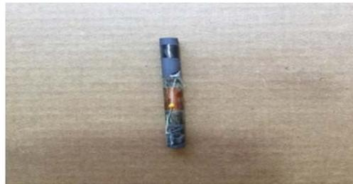
Fig. 2. The resonant circuit
