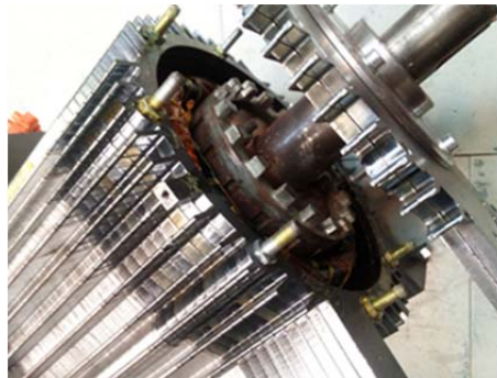
Fig. 9. Installation rotor into stator
