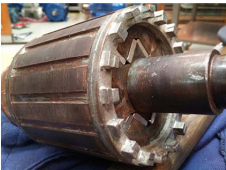
Fig. 7. Rotor after permanent magnets installation
