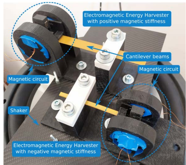
Fig.5. Dual system of electromagnetic energy harvesters on laboratory test-stand
