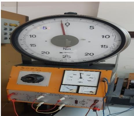
Fig.13. Load torque and corresponding speed for V/f=100/50
