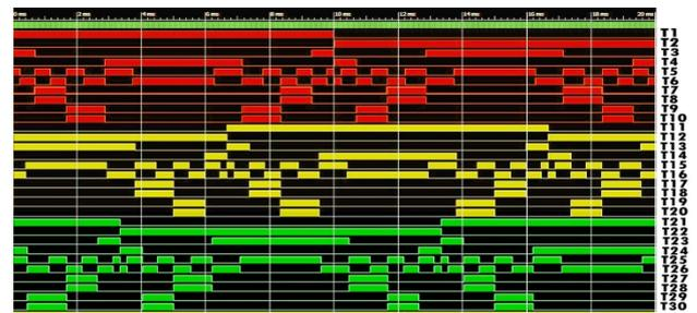
Fig.5. 3E Spartan MLI control signals wit corresponding switching states
