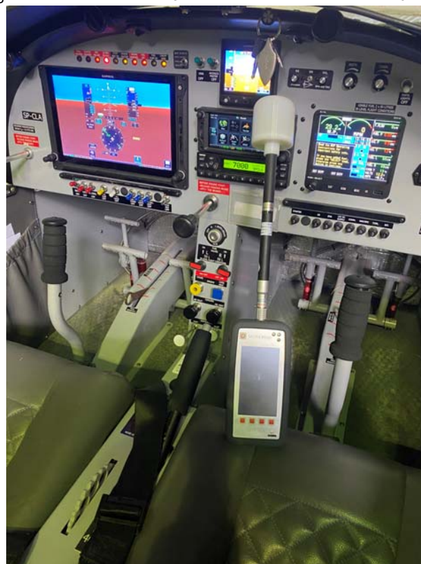
measuring probe, installed in the Aero AT3 aircraft.
