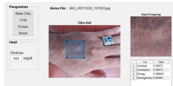
Fig.8. The results of data testing using the GLCM-Artificial Neural Network (ANN) method in the GUI program.
