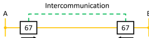
Fig.4. Schematic of line protection using directional protectors.
