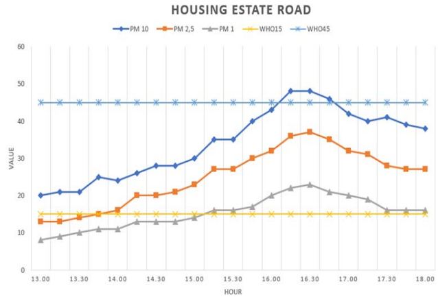
Fig. 4. Particulate matter levels for a residential road
