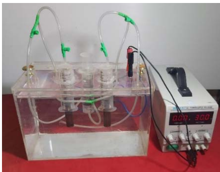
Fig. 1. Seawater electrolysis equipment
