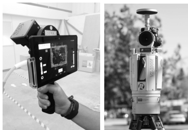
Fig.2. Mobile and Terrestrial laser scanners
