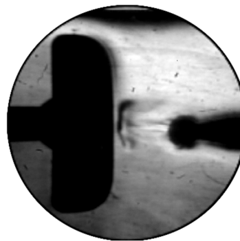
Fig. 4. EHD motion image obtained by the described method, for FR3 TiO 2 sample
