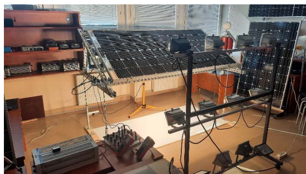
Fig. 4. Test stand in one of the configurations, module mounting height 120 cm, inclination angle 30°.
