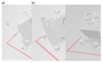
Fig. 8. Scanning results of the cube a) scan result without markers b) scan result of the cube with markers and additional normals
