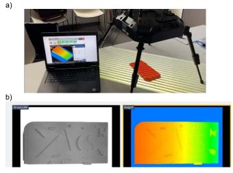
Fig. 5. Testing with white structured light (a) test stand (b) selected test results
