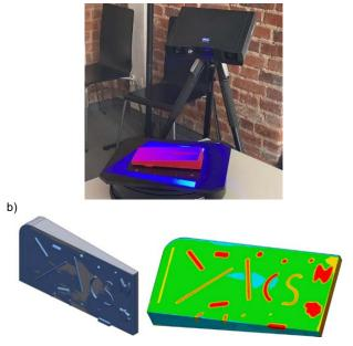
Fig. 4. Testing with blue structured light (a) test stand (b) selected test results
