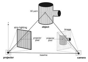
Fig. 1. Structured light scanning method Fig. 2.
