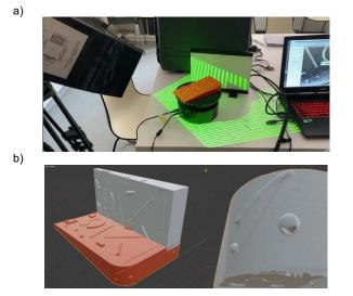
Fig. 6. Testing with green structured light (a) test stand (b) selected test results
