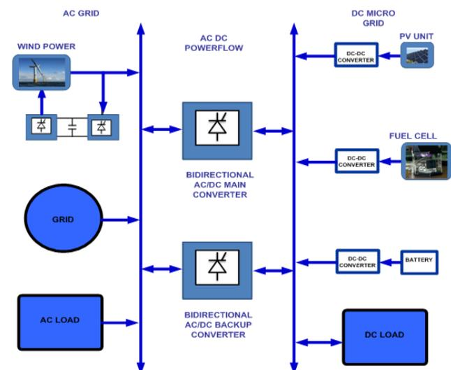
Fig.1. Typical RE based Microgrid System
