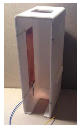
Fig. 2 Structure of the measurement capacitor, and the housing
