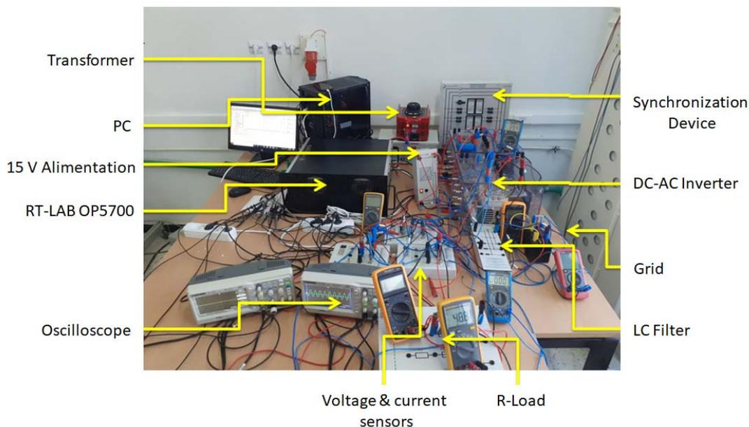
FIG. 8. Experimental test bench of a single-phase single-stage grid connected PV system
