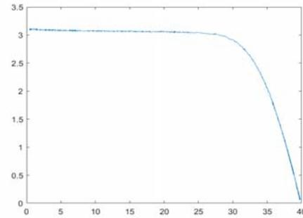
Fig. 4. Experimental I-V characteristic for a temperature of 40°C and a solar irradiance of 574W/m<sup>2</sup>
