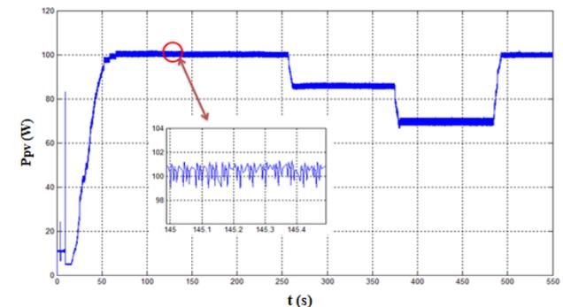
Fig. 14. Power of the PV panel
