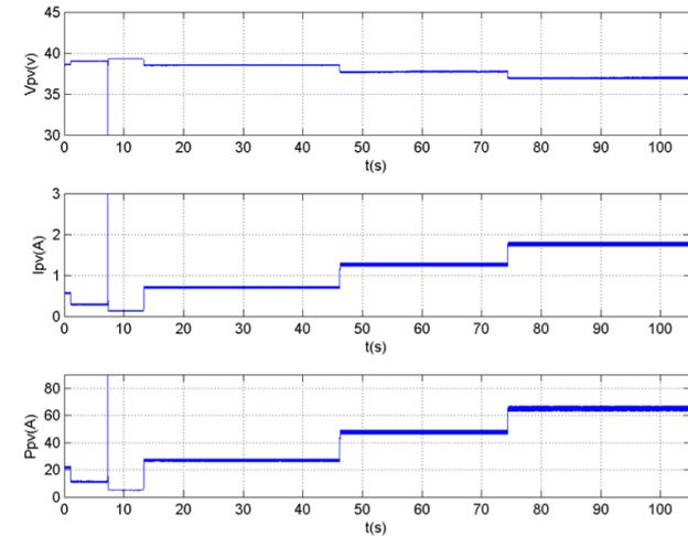
Fig. 10. Voltage, current and power of the PV panel
