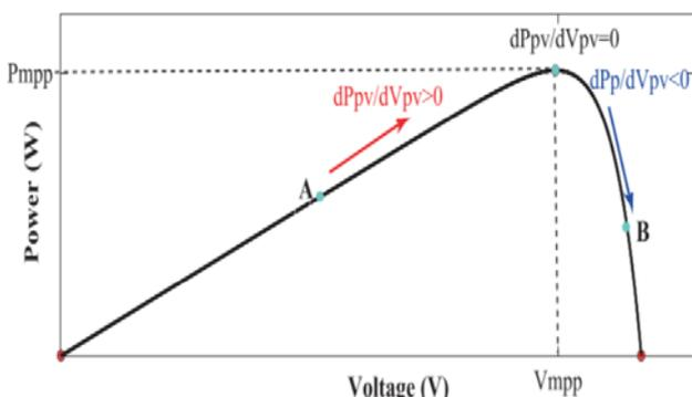
Fig. 7. Basic principle of P&O-MPPT method [20]
