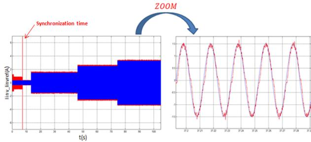
Fig. 9. Inverter current and its reference
