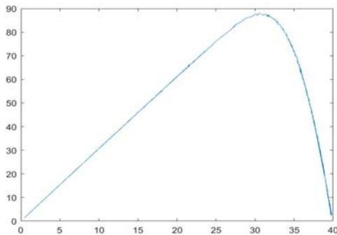
Fig. 5. Experimental P-V characteristic for a temperature of 40°C and a solar irradiance of 574W/m<sup>2</sup>
