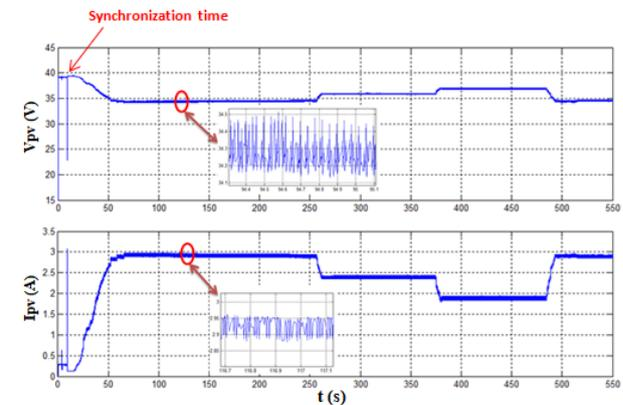
Fig. 13. Voltage and current of the PV panel
