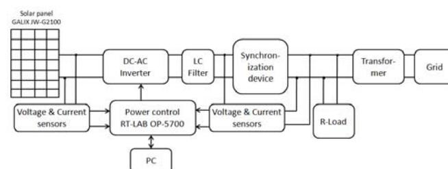
Fig.1. Single-phase single-stage grid connected PV system
