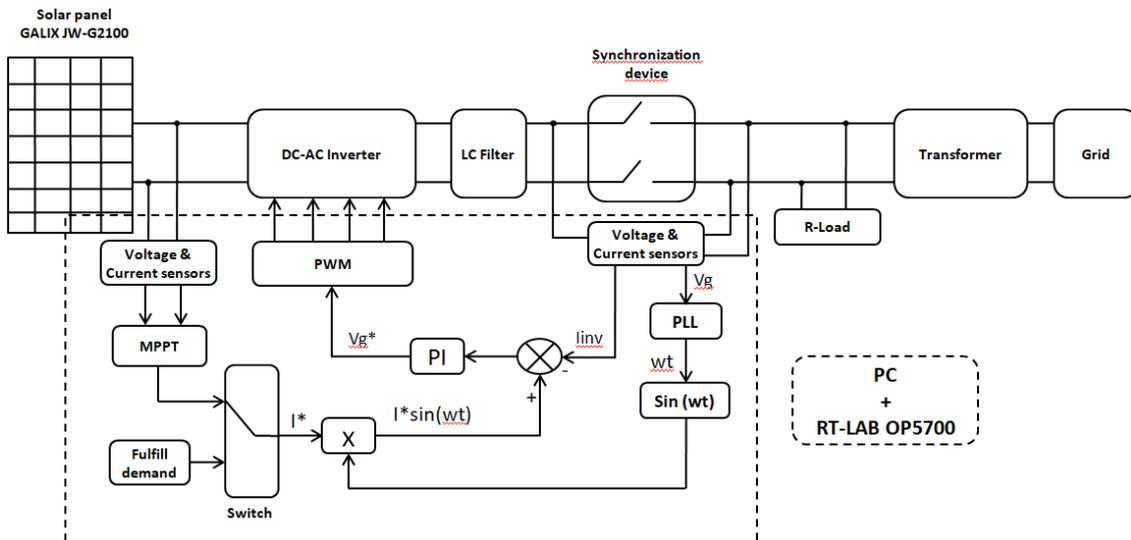
Fig.6. Injected power control of single-phase single stage grid connected PV system
