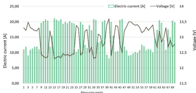
Figure 10. Current consumption (A) and voltage drops (V) when performing reversals
