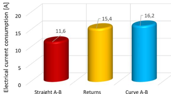
Figure 11: Current consumption of the automatic navigation system
