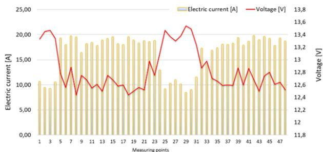
Figure 9. Current consumption (A) and voltage drops (V) during travel along the A-B curve line
