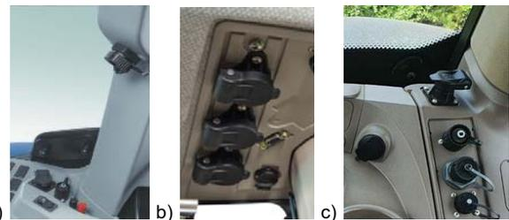
Figure 1. Power outlets in the tractor cab: a) New Holland t7 series, b) Fendt, c) John Deere [10- 12]
