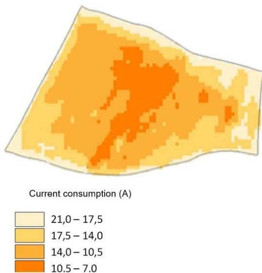
Figure 13. Spatial distribution of current increase in the installation of an automatic navigation system over an area of 26 hectares
