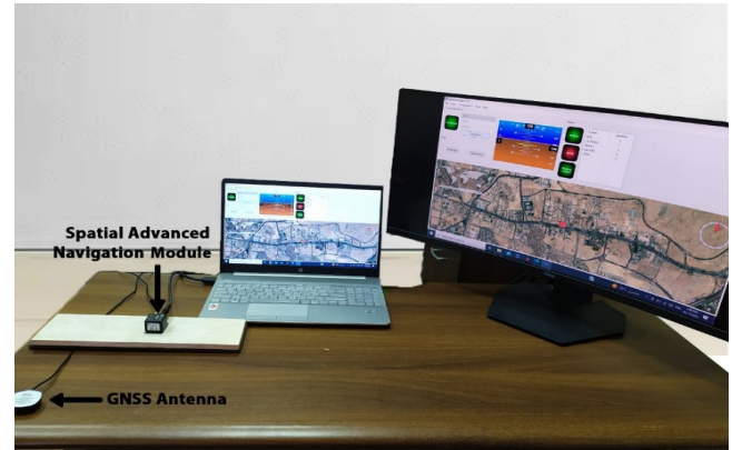
Fig. 6. Collecting static data setup in laboratory conditions.
