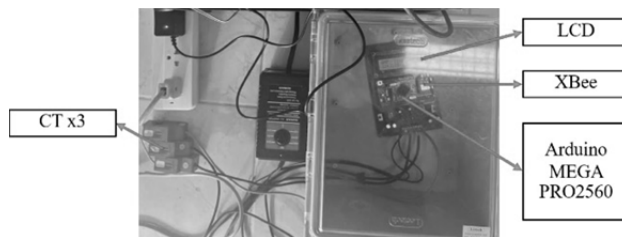
Fig. 3. A wireless electric current level detector.
