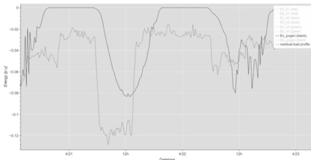
Fig. 3. Daily characteristics of an active energy generated in PV installation and a daily profile of residual active energy in 15-minute intervals in the considered factory on selected Saturday
