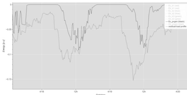
Fig. 2. Daily characteristics of an active energy generated in PV installation and a daily profile of residual active energy in 15-minute intervals in the considered factory on selected working day - Wednesday
