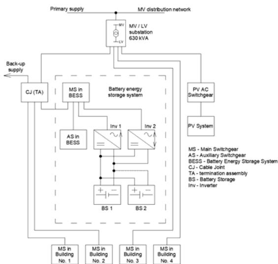
Fig. 1. The connection diagram concerning an internal electric power grid in the considered industrial enterprise.
