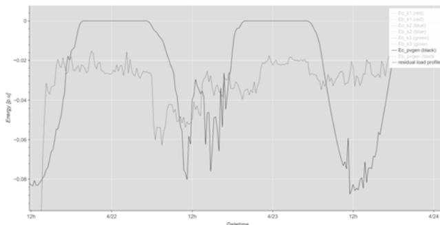
Fig. 4. Daily characteristics of active energy generated in PV installation and a daily profile of residual active energy in 15-minute intervals in the considered factory on selected Sunday
