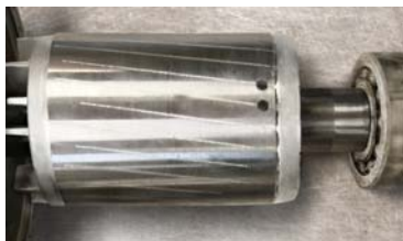
Fig.5. Malfunction of the rotor winding
