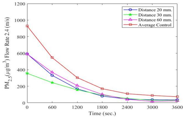
Fig. 7 Results of PM<sub>2.5</sub> Particulate Matter Removal at Varied Electrode Distances.
