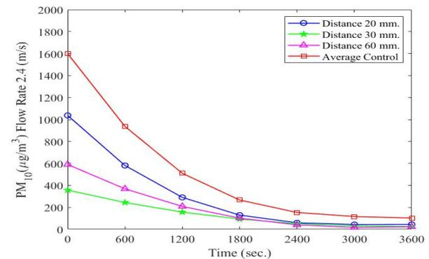
Fig. 9 Results of PM<sub>10</sub> Particulate Matter Removal at Varied Electrode Distances.
