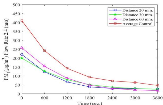
Fig. 5 Results of PM1 Particulate Matter Removal at Varied Electrode Distances.
