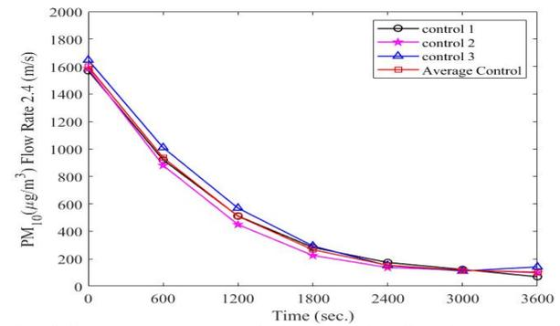
Fig. 8 Cumulative Findings Pertaining to the Quantification of PM<sub>10</sub> Particulate Matter in the Control Apparatus.
