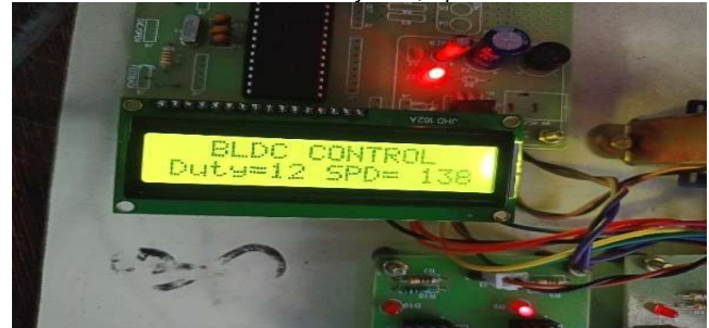
(d) BLDC motor ( 1 . 5 K R P M ) CONTROL with DC-DC boost converter Duty = 12, Speed = 138 RPM
