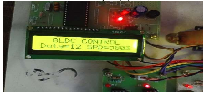
Fig. 12 Description of Hardware setup of proposed system Non-linear controller (ANF-SMC) with BLDC motor speed of 1500 RPM and used converter.
