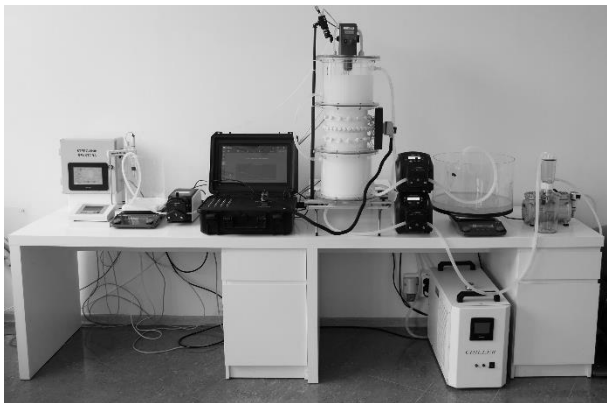
Fig. 6. A process demonstrator equipped with a reactor for the crystallization process
