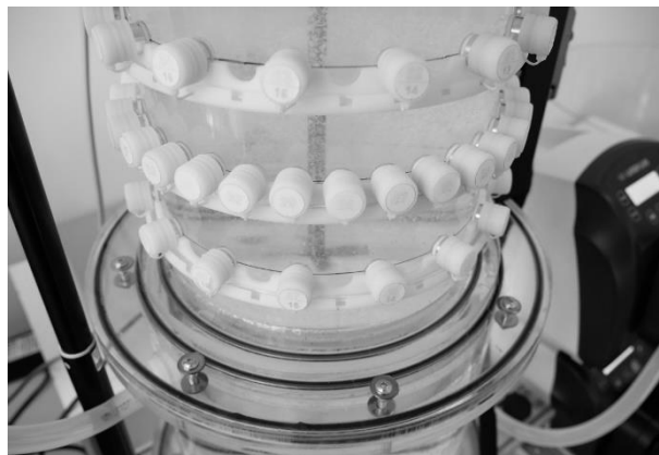
Fig. 7. Precipitated calcium carbonate inside the reactor with 64 transducers 300kHz frequency
