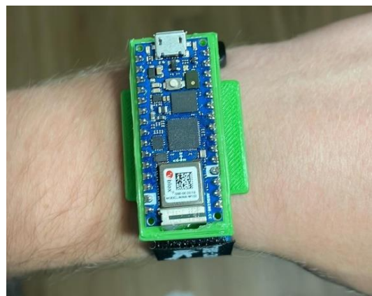
Fig. 1. Personal fall detector on the wrist. Prototype version (photo: M. Czumak).
