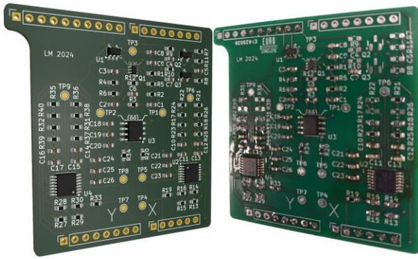
Fig.4. Rendering of PCB design and the assembled board
