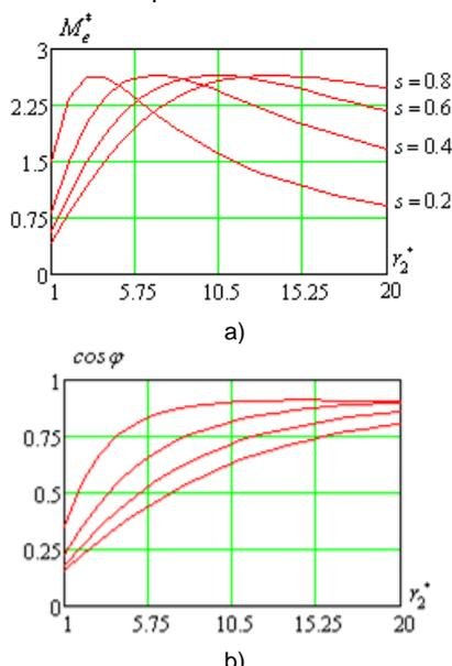
Fig. 2. Dependencies of the driving electromagnetic torque of the WRIM (a) and the power factor  $\cos\varphi$  (b) from the relative value of the resistance of the rotor phases together with the rheostat for different slip values
