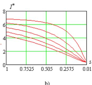
Fig. 1. Starting characteristics of electromagnetic torque (a) and stator current (b) at different values of rheostat resistance in the rotor circuit
