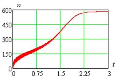
Fig. 3. Transient process to the steady-state speed of the WRIM rotor with the rheostat turned on at the value of the rheostat resistance  $r_p = 4r_2$
