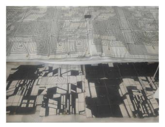
Fig. 5. Prototype of the heating mat in actual dimensions of  $200 \times 90$  cm. Top layer - heating elements, bottom layer - connections and power lines.
