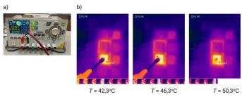
Fig. 3. The heating layer of the mat under the pressure: a) power supply, b) thermograms
