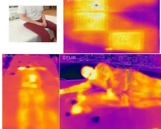
Fig. 9. Testing of prototype heating layer under human load: a) test course, b) thermogram c) reality tests.
