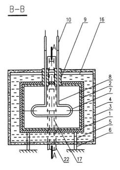
Fig. 2. Transversal cross section of the resonator with the B-B plane – the designations of the elements are the same as in Fig. 1.
