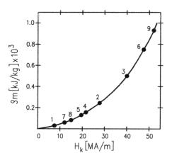
Fig. 4. Dependence of the massive energy density  $\rho_m$  on the critical field intensity  $H_k$  for the superconductors under consideration, point numbers denote numbers of lines in Tab. 1
