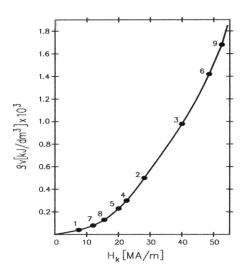
Fig. 3. Dependence of the volumetric energy density  $\rho_V$  on the critical field intensity  $H_k$  for the superconductors under consideration, the point numbers denote the numbers of lines in Tab. 1
