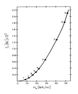
Fig. 5. Dependence of the total energy in the  $E_r$  resonator on the critical field intensity  $H_k$  of the superconductors used to make it, the numbers of points denote the numbers of lines in Tab. 1
