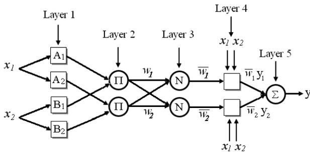
Fig. 5. Equivalent ANFIS architecture
