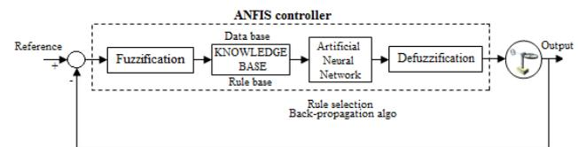
Fig. 3. Block diagram of the ANFIS control scheme.
