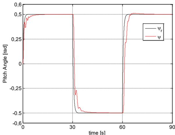
Fig. 9. TRMS pitch angle control system evolution trajectories with square input reference with ANFIS controller.
