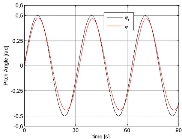
Fig. 11. TRMS pitch angle control system response with sinusoidal input reference with ANFIS controller.
