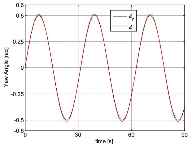
Fig. 12. TRMS yaw angle control system response with sinusoidal input reference with ANFIS controller.
