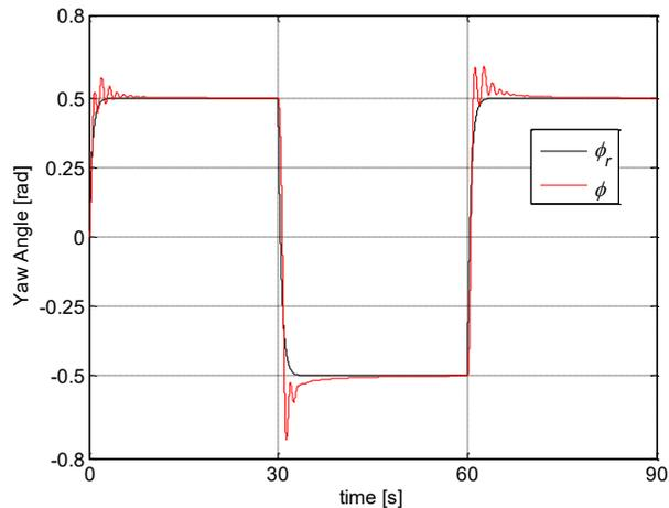
Fig. 10. TRMS yaw angle control system evolution trajectories with square input reference with ANFIS controller.
