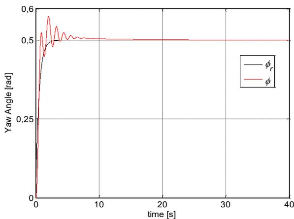
Fig. 8. TRMS yaw angle control system response with step input reference with ANFIS controller.
