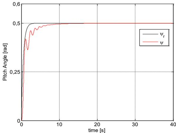
Fig. 7. TRMS pitch angle control system response with step input reference with ANFIS controller.
