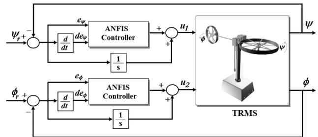
Fig. 6. Block diagram of the proposed ANFIS control scheme of TRMS.
