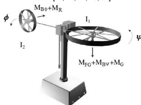
Fig. 1. Rotor multi-input-output System (TRMS).
