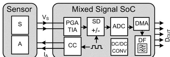
Fig. 1. Generalized structural diagram of the sensor device
