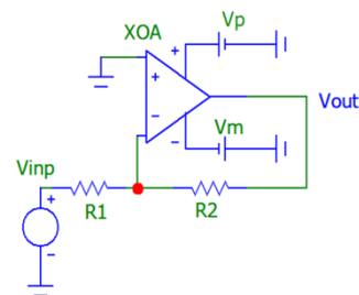
Fig. 7. SPICE scheme of the inverting amplifier model
