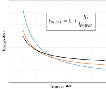
Fig. 9. Dependence of the delay time on the supply current
