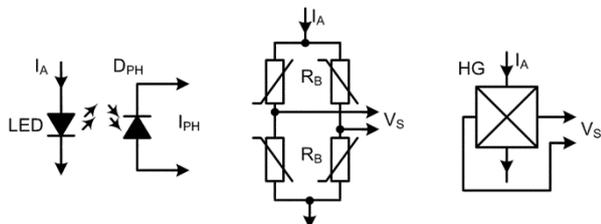
Fig. 2. Primary transducers of the sensor device
