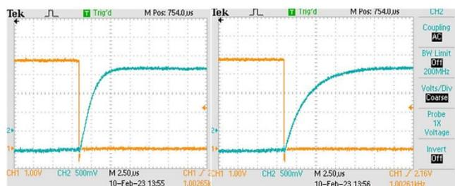
Fig. 6. Oscilloscope of PGA output voltage increase in High Power mode (left) and Low Power mode (right)
