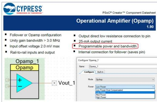
Fig. 5. Specification and Opamp PSoC configuration window
