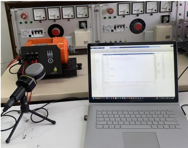
Fig. 1. Test bench for acquiring motor noise.
