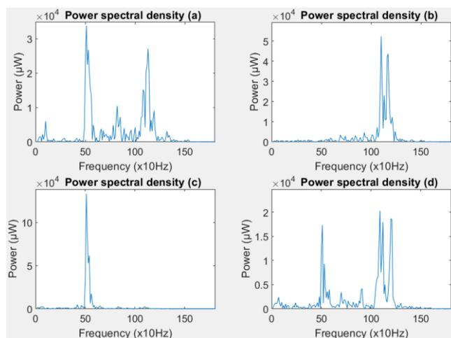
Fig. 6. STFT of motor noises.
