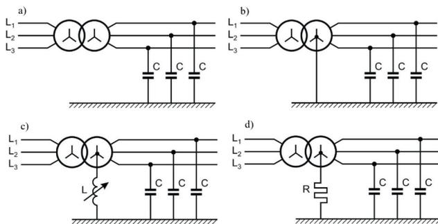
Fig. 1. The method of work of a neutral point of the grid in the National Power System: a) insulated, b) effectively grounded, c) grounded by reactance, d) grounded by resistor
