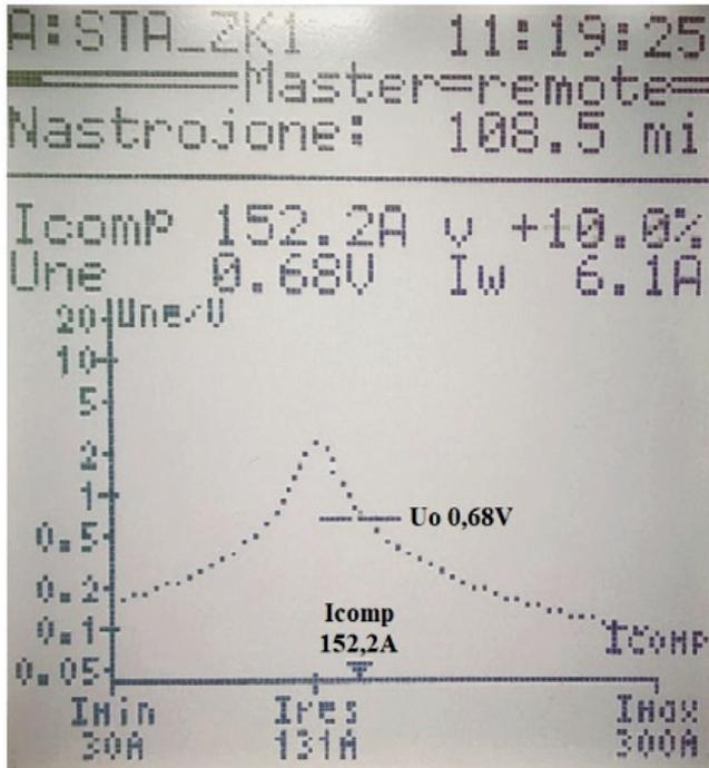
Fig. 13. A view of DP regulator with a resonance curve
