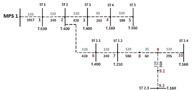
Fig. 9. Single line diagram of the medium-voltage line 7 powered by the main power supply station 1
