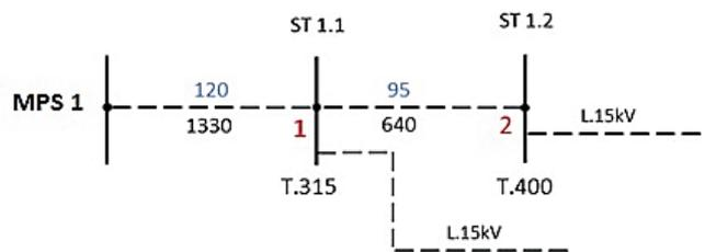
Fig. 8. Single line diagram of the medium-voltage line 13 powered by the main power supply station 1: ST – transformer station along with its number, T.315 – 315 kVA transformer, 120, 95 – wire diameter, 1330, 640 length of the sections, 1, 2 grid nod
