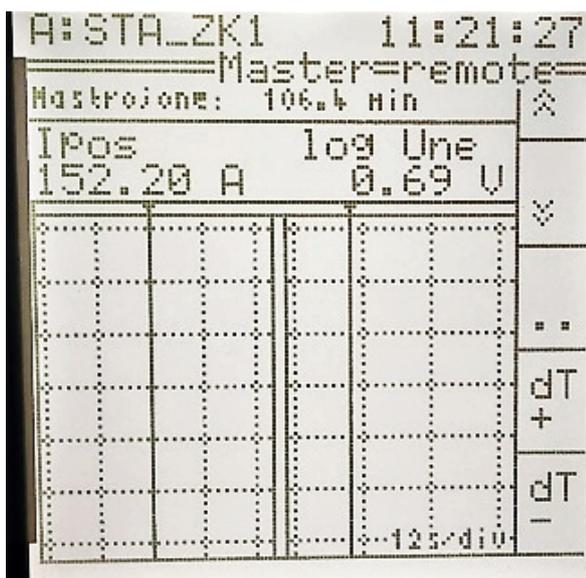
Fig. 11. A view of a regulator display with a current position of a choke and  $U_{ne}$  ( $U_0$ ) voltage logarithmically within the range of three decades, which corresponds to the range 0,1 ...100V, pace of change registration (refreshing) 12 s/scale
