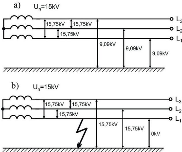
Fig. 3. The value of phase and line-to-line voltages in the medium-voltage grid; a) normal work, b) work with grounded phase  $L_1$  [2]
