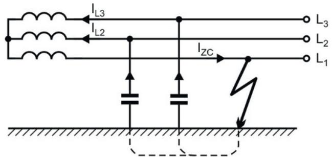
Fig. 4. Direction of flow of capacity current  $I_{zc}$  in a medium-voltage line in ground fault of phase  $L_1$  [3]
