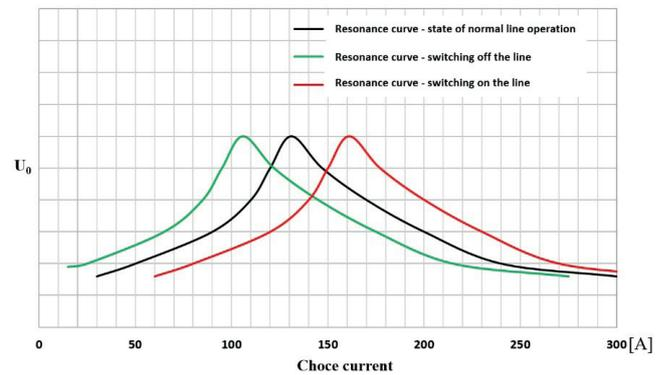
Fig. 12. Resonance curves depending on configuration of a medium-voltage grid
