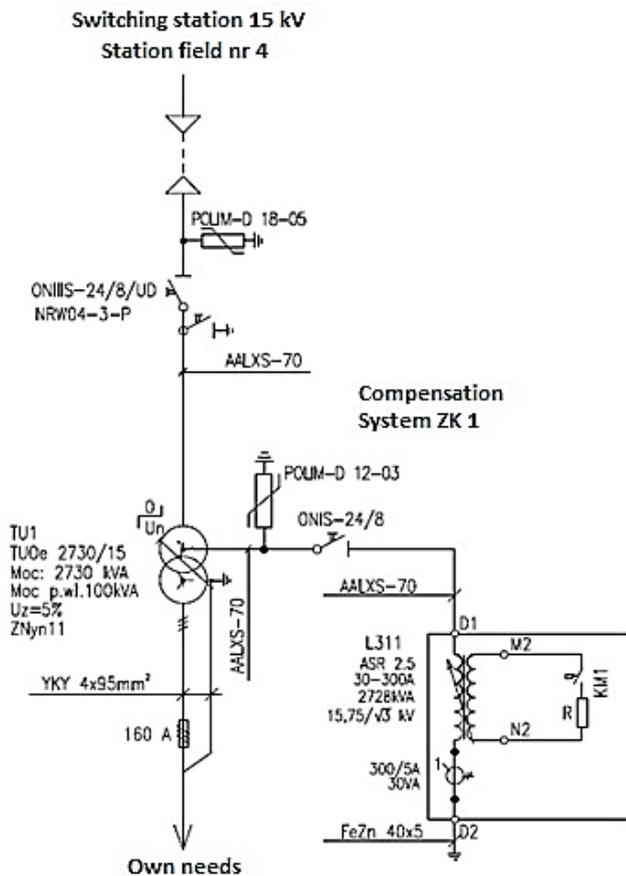
Fig. 14. Diagram of follow-up compensation for the bay 4 and 41 for both sections in 15 kV medium-voltage switching station
