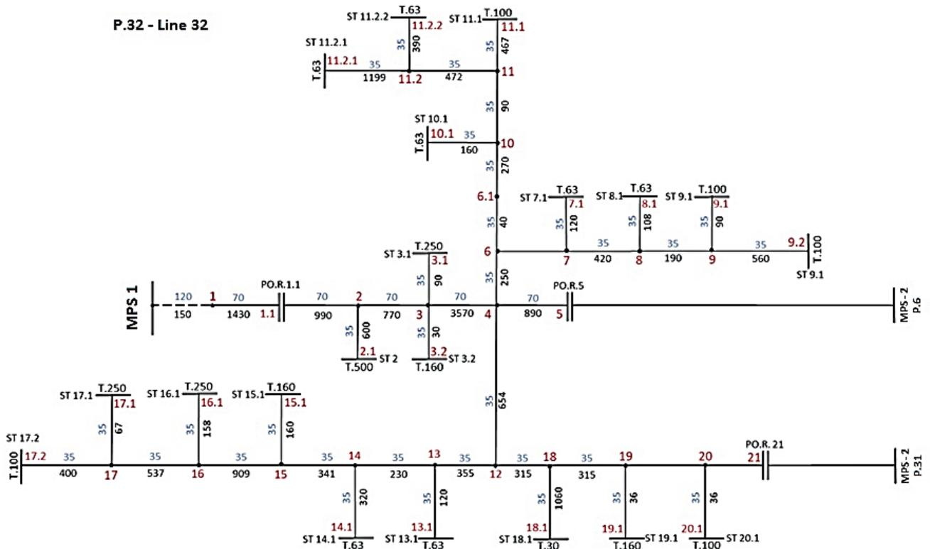
Fig. 10. Single line diagram of the radial line 32 with radio-controlled disconnectors inside the grid: PO.R.1.1 – radio-controlled disconnecting point
