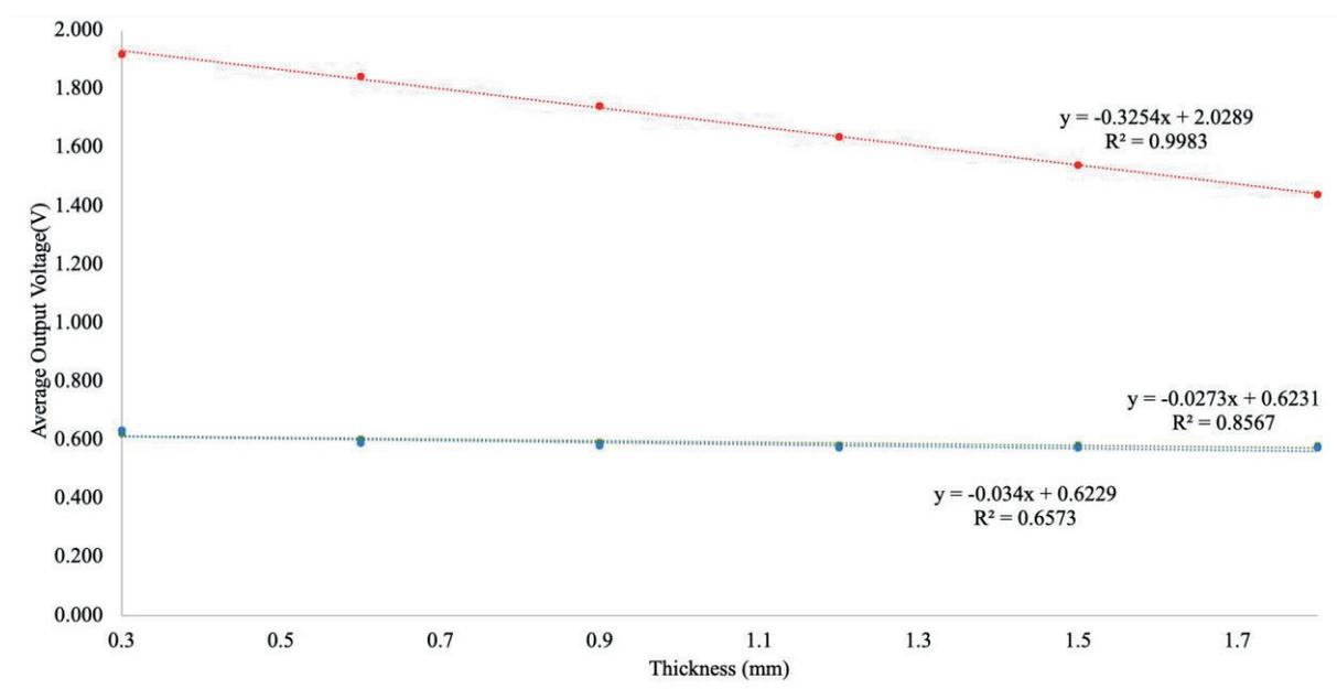
Fig. 3: Sensing performance for red transparent PVC sheet with RGB LED light Source
