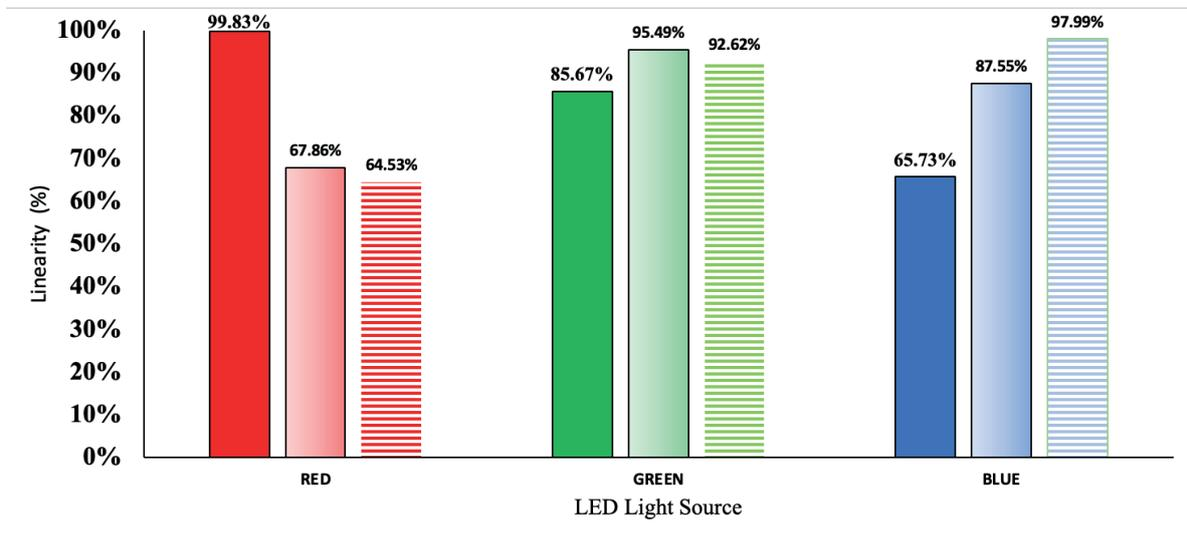
Fig. 7: Linearity comparison for the three transparent PVC sheets
