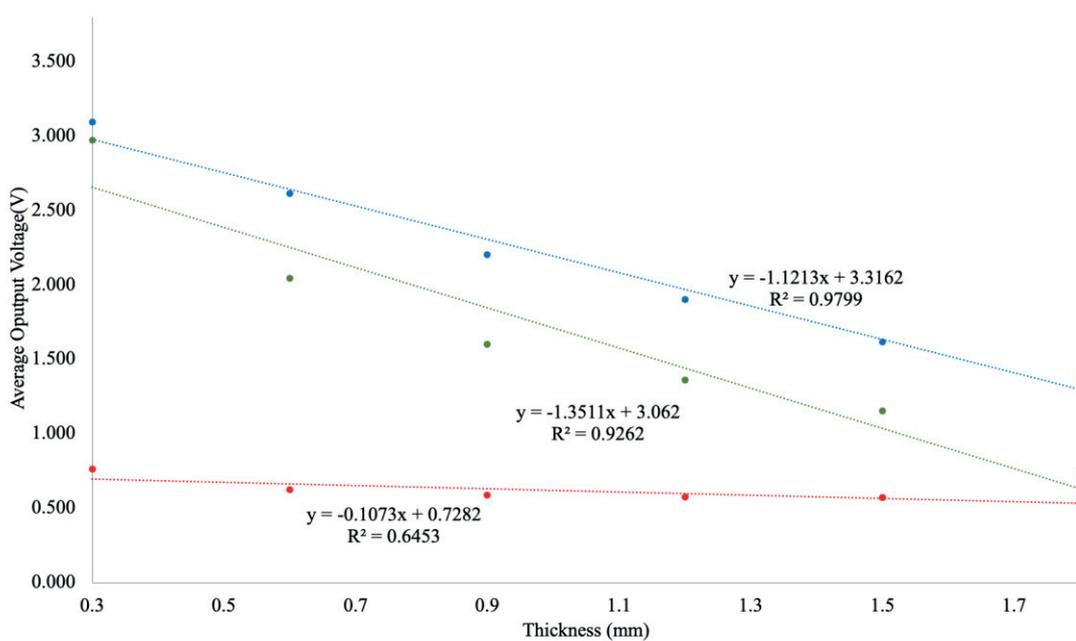
Fig. 5: Sensing performance for blue transparent PVC sheet with RGB Light Source
