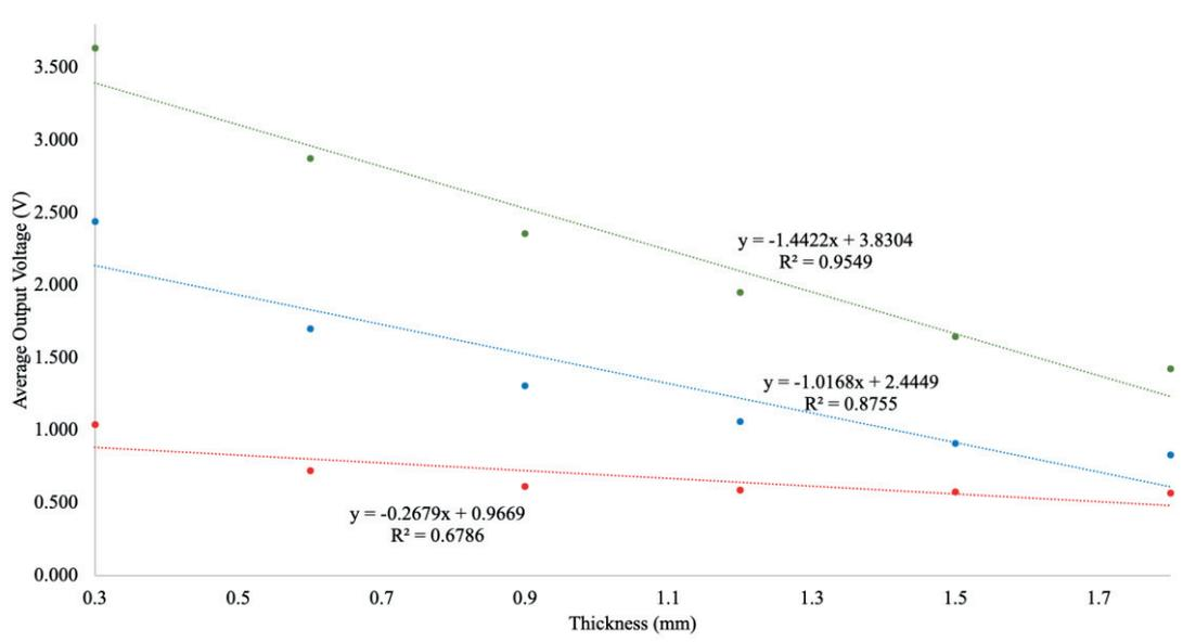
Fig. 4: Sensing performance for green transparent PVC sheet with RGB Light Source
