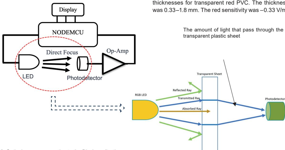
Fig. 2. Optical sensor connection to the Blynk application
