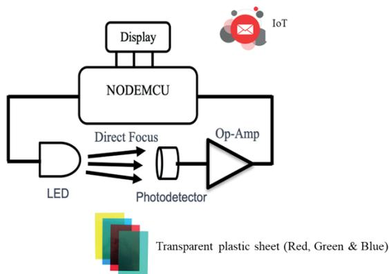
Fig. 1. Sensing Mechanism for thickness measurements
