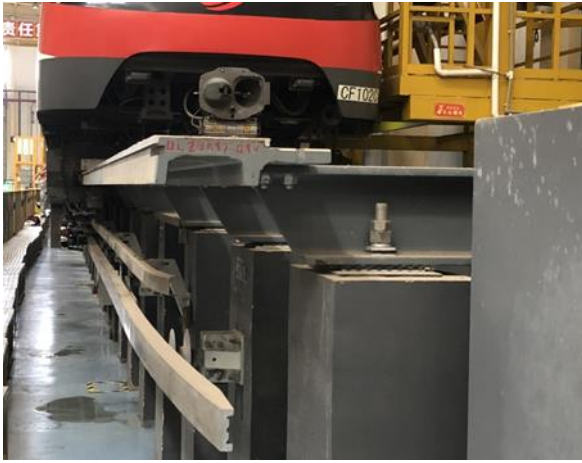
Fig. 14. Changsha Maglev train depot. Guideway with aluminum plate at the top and two contact rails. Photo taken by the author.
