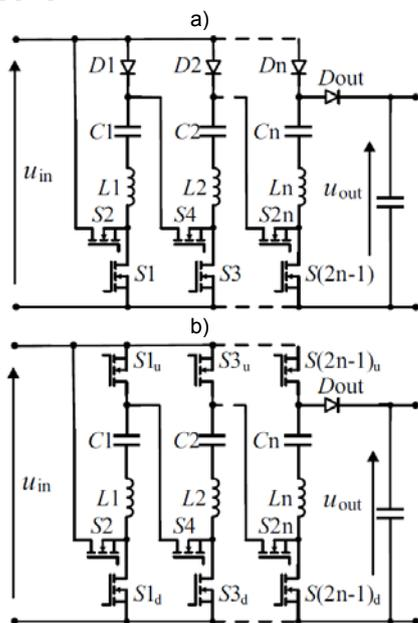
Fig.1. DC-DC converter in the topology of: (a) basic Resonant Switched-Capacitor Voltage Multiplier (SCVM), (b) Synchronous Resonant Switched-Capacitor Voltage Multiplier (SYSCVM) [9]
