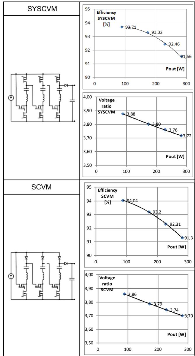
Fig.8. Experimental results of the SYSCVM. Results of measurements of efficiency and the voltage ratio versus power of the SYSCVM and SCVM converters.  $U_{in} = 30\text{ V}$
