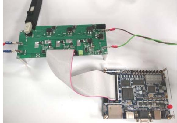
Fig.4. Experimental setup of the SYSCVM with an FPGA-based pulse generator (DE zero board)
