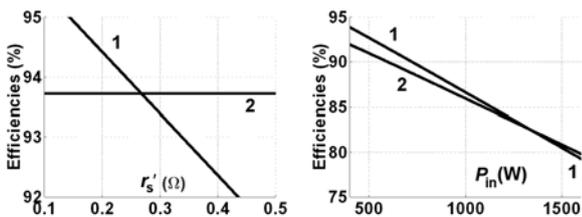
Fig.3. Efficiencies of SYSCVM and SCVM as a function of: (a)  $r_S'$  at  $P_{in} = 200$  W, (b)  $P_{in}$  at  $r_S' = 40$  m $\Omega$ . 1 - SYSCVM, 2 - SCVM. Common parameters:  $n = 3$ ,  $U_{in} = 30$  V,  $T_{SI}/T_S = 0.5$  (zero dead-time),  $r_S = 100$  m $\Omega$ ,  $U_{DS} = 1.1$  V,  $f_S = 109.8$  kHz,  $\Delta W_{sw} = 10$   $\mu$ J. Calculations based on (1) and (3)
