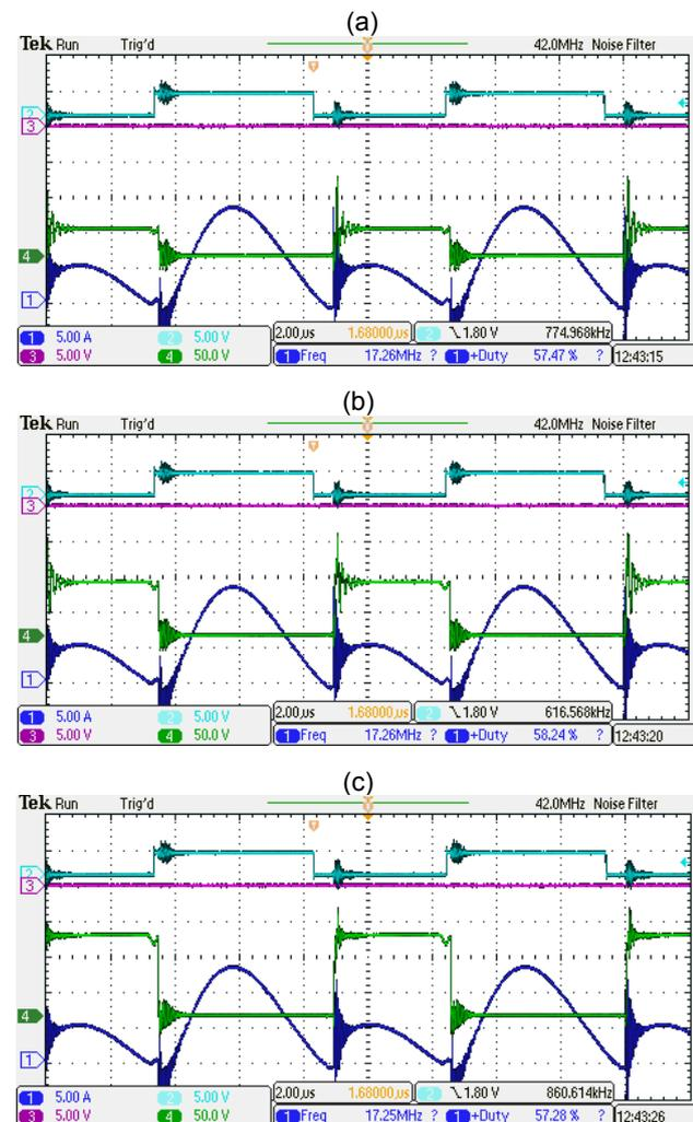
Fig.7. Experimental results of the SYSCVM. Waveforms of the input current (1) and voltage on the upper switch (4): the  $S_{1u}$  (a), the  $S_{2u}$  (b), the  $S_{3u}$  (c).  $U_{in} = 40\text{ V}$ . Channel (2) displays control signal of lower charging transistors
