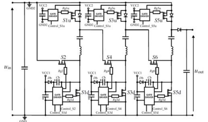
Fig.5. The proposed gate driver system in the SYSCVM
