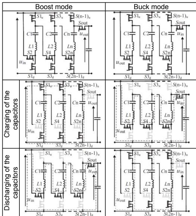
Fig.9. A bi-directional buck-boost converter and its operation modes
