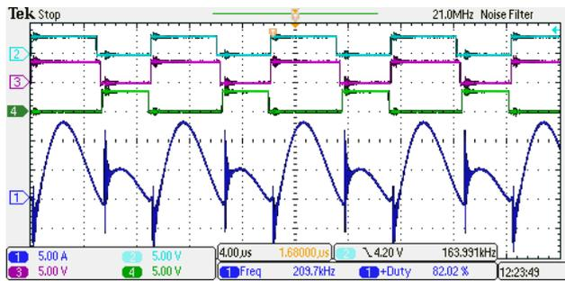
Fig.6. Experimental results of the SYSCVM. Waveforms of the input current (1) and control signals of groups of transistors: lower charging transistors (2), upper charging transistors (3), discharging transistors (4).  $U_{in} = 40\text{ V}$ ,  $P_{out} = 200\text{ W}$
