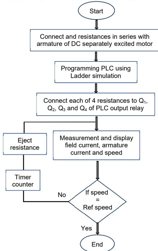
Fig. 6. Flowchart of armature resistance based PLC.
