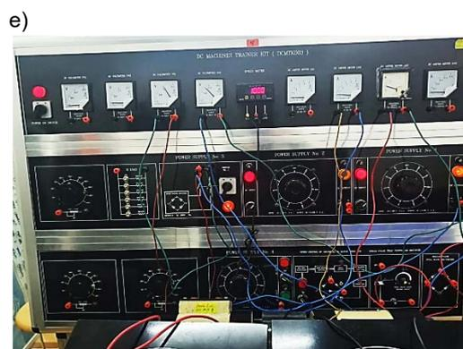
Fig. 7. Practical circuit for speed control of separately excited DC motor.
