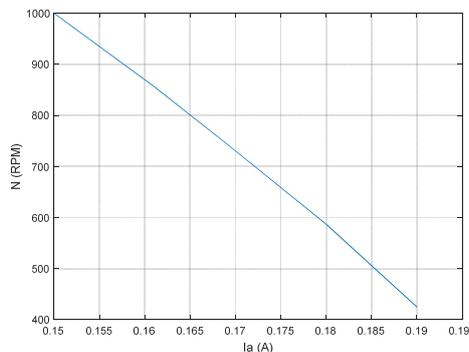
Fig. 8. Speed of DC motor vs armature current
