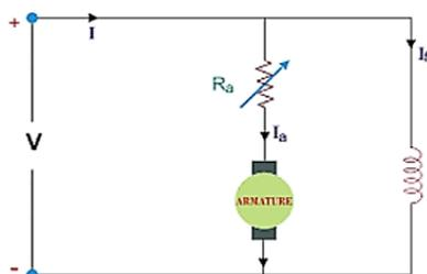
Fig.2. Armature control of DC motor
