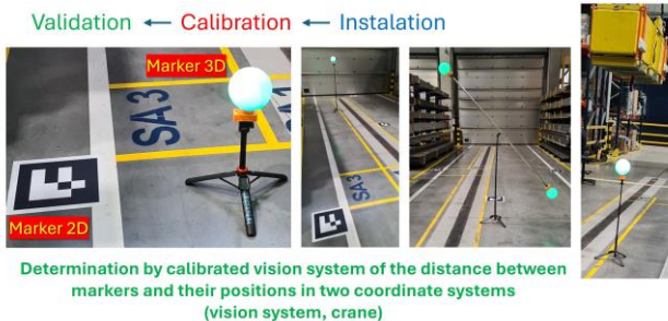
Fig. 10. Commissioning of the vision system on the target measurement stand - validation
