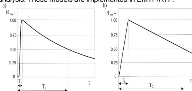
Fig. 1. Models of lightning stroke current: a - Heidler's model, b - model proposed by CIGRE [4,10,18,19]
