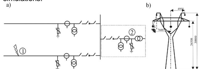
Fig. 2. a - single line diagram of the part of the electrical power system of 220 kV: 1 - point of lightning discharge and simulation of overvoltages at the tower, 1,2 - the points for simulations of overvoltages, b - basic dimensions of tower of 220 kV [28]
