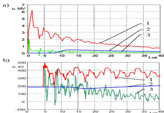
Fig. 4. Overvoltages at the part of the electrical power system of 220 kV (Fig. 2) simulated during lightning stroke to the shielding conductor (33.3 kA) in the point 1 of line: a - overvoltages at the tower (point 1), b - overvoltages between phase conductor and earth (point 2): 1 - CIGRE model for the first positive discharge, 2,3 - Heidler's model (2 - first positive stroke, 3 - subsequent negative discharge)
