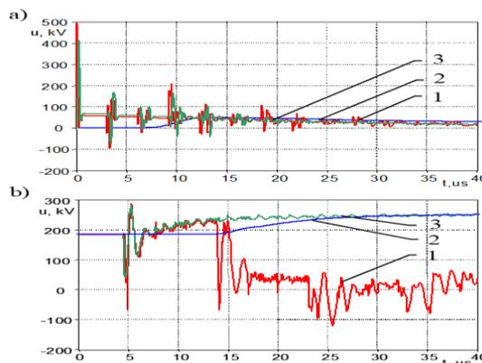
Fig. 5. Overvoltages at the part of the electrical power system of 220 kV (Fig. 2) simulated during lightning stroke to the phase conductor (14.08 kA) in the point 1 of the line: a - overvoltages at the tower (point 1), b - overvoltages between phase conductor and earth (point 2): 1 - CIGRE model for the first positive discharge, 2,3 - Heidler's model (2 - first positive stroke, 3 - subsequent negative discharge)
