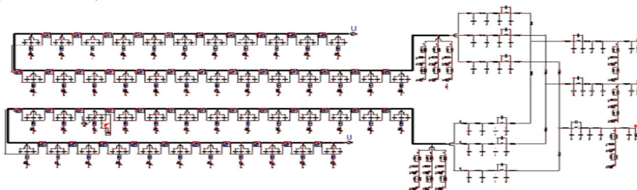
Fig. 3. Model of the part of electrical power system presented in Figure 2 used in simulations of lightning overvoltages prepared in EMTP/ATP
