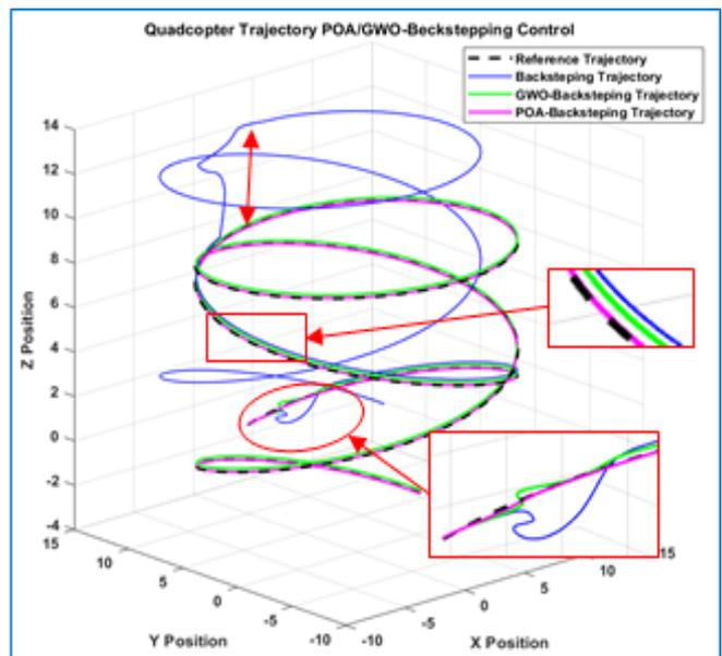
Fig. 9. 3D tracking path of Quadcopter in windy environment: Helical path
