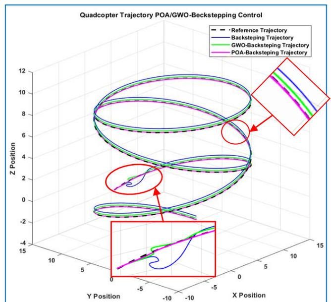
Fig. 5. 3D Quadcopter Tracking Trajectory: Helical Path
