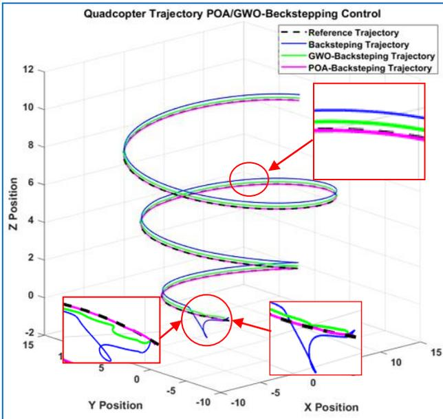
Fig. 3. 3D Quadcopter Tracking Trajectory: Conical Path
