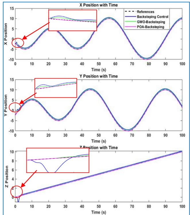
Fig. 2. Result of tracking conical path in Z, Y and X axes
