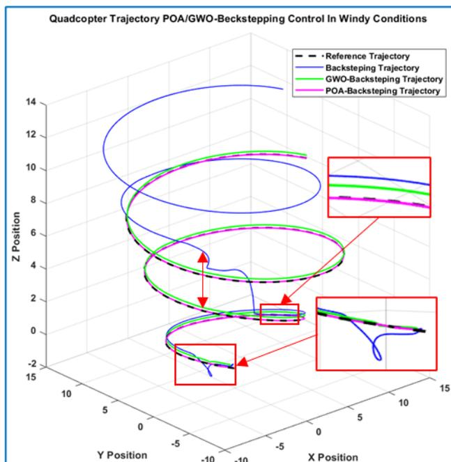
Fig. 8. 3D tracking path of Quadcopter in windy environment: Conical path
