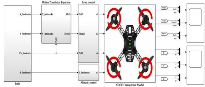
Fig. 1. Simulation bloc for 6DOF Quadcopter using backstepping controller [18].
