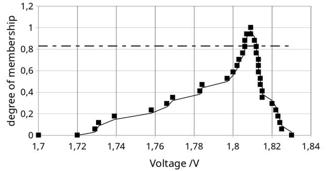
Fig. 4. The membership function of the output voltage, the horizontal dashed line at the level  $\alpha = 0.83$  indicates the cut at the level  $\alpha' = t^{[-1]}(\frac{1}{n}t(\alpha))$
