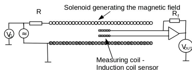
Fig. 2. Measuring circuit for calibration of induction field meter
