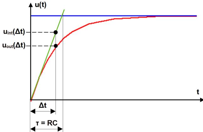
Fig. 2. Unit step function  $1(t)$  - blue line, ideal integration - black line and exponential rise at the output of the passive RC integrator - red line.
