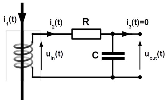
Fig. 1. Electrical circuitry by measurement with the current probe.
