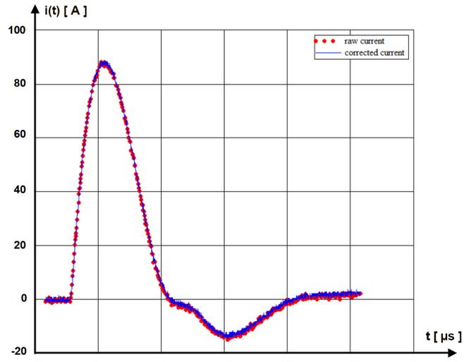
Fig. 8. Raw and corrected current captured with probe model 1423.
