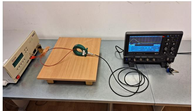
Fig. 3. Measurement set up with probe model 110A.
