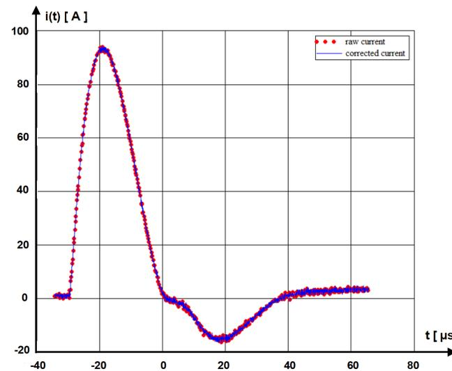
Fig. 7. Raw and corrected current captured with probe model 6600.
