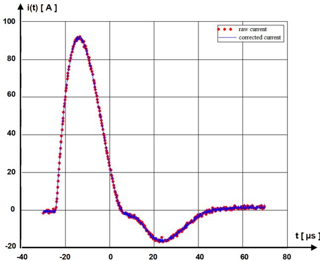
Fig. 6. Raw and corrected current captured with probe model 110A.
